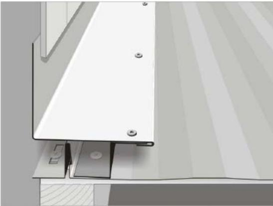
Fig. 17 Standard Sidewall attaches to z-flashing with screws
